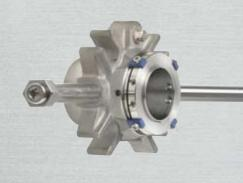
Rubber materials Different combinations of O-rings in shaft seals and in the pump are possible in order to adapt to the specific application. Special rubber types such as FXM (Flouraz®), FFKM (Kalrez®), and HNBR are available where the liquid may damage standard O-ring materials such as EPDM, FKM and Viton®.
